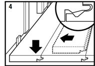
Slide panel into space horizontally and slot into profile. Use these modified planks under doorframes, radiators, cabinet fronts, etc. Use the pull bar to slide the planks where needed.
