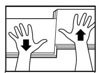
DISASSEMBLING: Disengage entire row by lifting up row delicately at an angle. To separate individual planks, leave them on the ground and then carefully slide the planks apart as illustrated.
