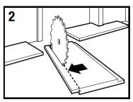
Remove the tongue side (see pictures above) on only the planks in the first row that face the wall to allow room for spacers.
