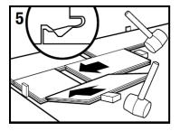
Use a 4"-6" piece at an angle to hold the tongue and the groove on the same plane, limit end-joint damage and ensure planks engage square. Tap end-joints with multiple taps, striking the tapping block evenly until end-joints close. NOTE: Tapping too hard or striking the tapping block unevenly can result in installation-related damage or peaking.
