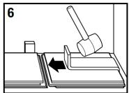
Fit the last panel in the row using a pull bar.
