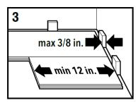
Always allow for 5/16" min to 3/8" max expansion at walls and around fixed objects. A transition strip is required when length or width of installed planks measures 40' and in doorways if plank direction changes.
