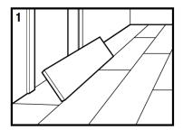
Some long edge joints cannot be installed using a  $20^{\circ}$  angle.
