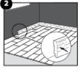
Inspect the final surface of the installed floor. Install vinyl skirtings against the wall but never attach the skirting to the floor itself. This method allows the floor to expand and/or contract under the skirting-board. Do not fill or cover the expansion joints with silicone or other kit.
