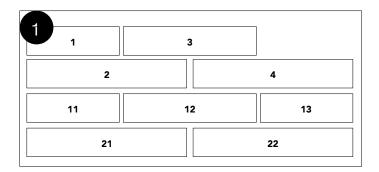
ESTABLISH STAGGER AND ALIGN TOOLS Products should be staggered in bricklaid pattern, stagger equal to half of a plank. Tools needed: planks, underlayment, spacers, rubber mallet, cutter.
