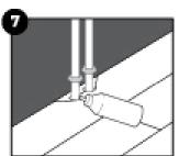
Then, using an appropriate PVC glue along the cut edges of the piece you cut out, glue the piece in place. Be sure no glue comes between the cut out piece and the subfloor. For a perfect finish around pipes, use pipe covers.
