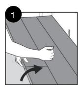
Separate the whole row by carefully lifting up and release the whole row.
