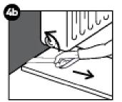
When sawing the panels make sure that the expansion gap under the door is 10mm. If you cannot lift the panel (e.g. under radiators), use the tapping block or pull-bar to tap the planks together.
