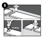
In rows where there is a pipe, make sure the pipe falls exactly in line with the short side of two planks. Take a drill bit with the same diameter as the pipe plus 16mm (0,63inch). Click the planks together on the short side and drill a hole centered on the joint between the two planks. Now you can install the planks.
